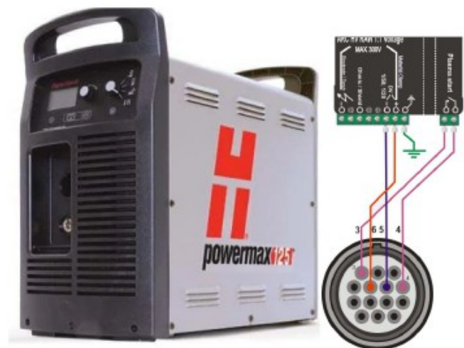
Connection of plasma sources with voltage divider 1:50 ( 20V MAX )
