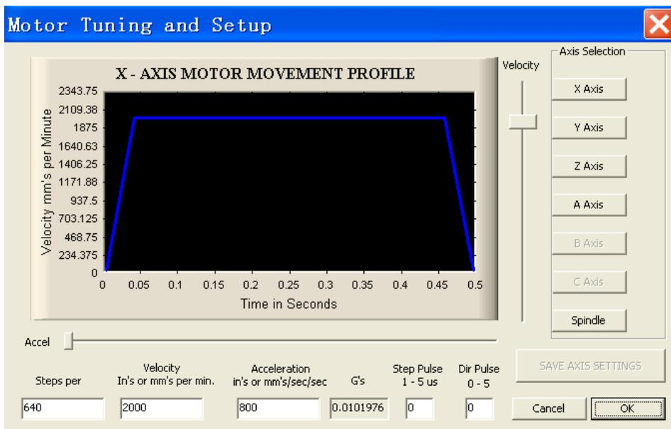
1、 **Steps per** This must be right. In the case of the stepping motor of 1.8 degree, **Steps per** the numerical= $360/1.8$ \*fine fraction/leadscrew pitch.
