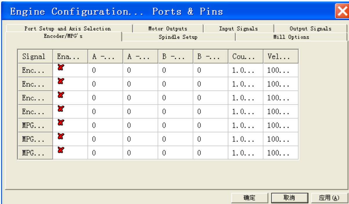
7、Chief axis settings. It should be noted that "pulse width modulation base" is based on each PC configuration. The system generate automatically. There are 2 kinds of spindle control, which can use the relay, and the 0-10 port to control.
